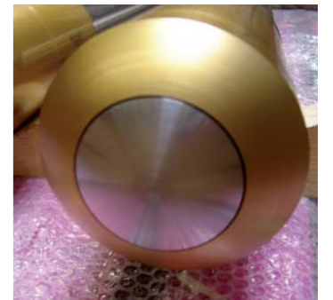
Piston head with tungsten carbide coating
