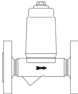
Condensate discharge temperature limiter
