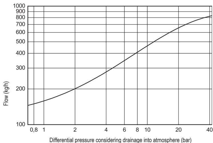
The capacity chart shows the maximum flow of hot condensate for the standard controller
