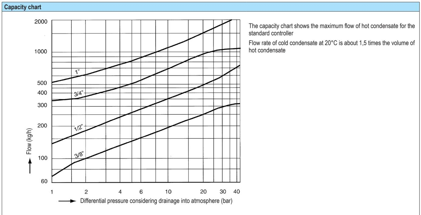
**Thermodynamic steam trap (High temperature steel)**
