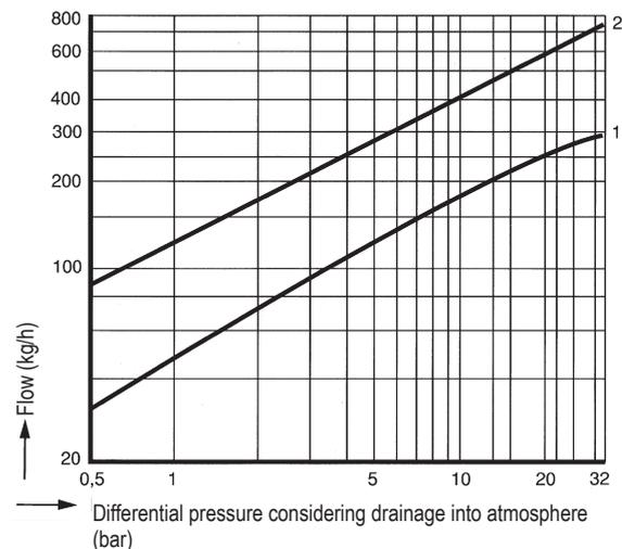
The capacity chart shows the maximum flow rates for controller.
