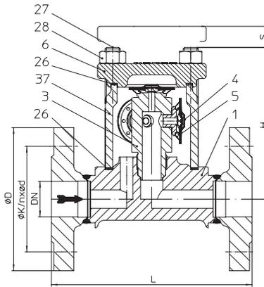
Fig. 616...1...4K2 (DN25) with 4 capsules, with flanges
