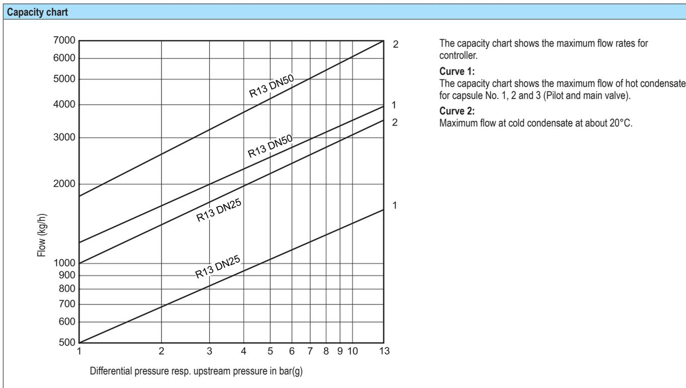
**Thermostatic steam trap with multi capsule for very high flow capacity (Forged steel)**
