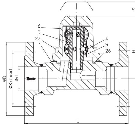
Fig. 616...1...6K2 (DN40-50) with 6 capsules, with flanges
