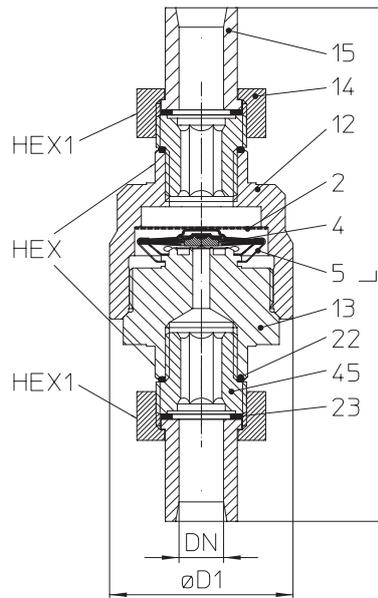
Fig. 614...5 union with butt weld ends
