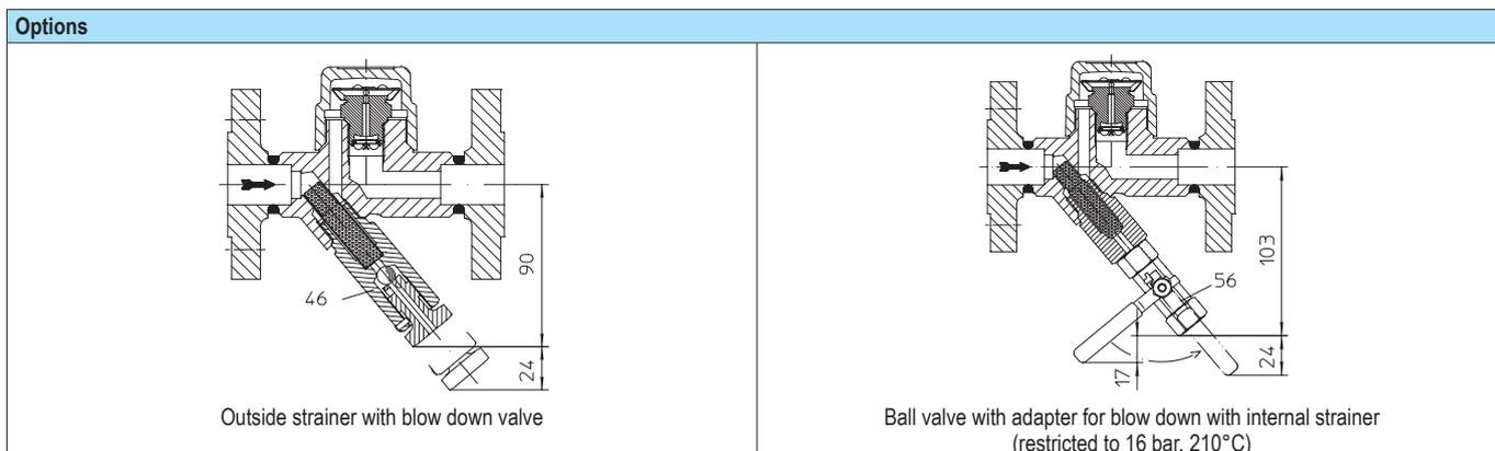
**Thermostatic steam trap for higher flow capacity (Forged steel, High temperature steel, Stainless steel)**
