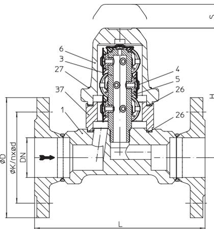
Fig. 616...1...10K2 (DN40-50) with 10 capsules, with flanges
