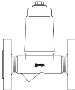
Condensate discharge temperature limiter
