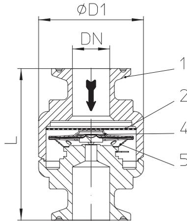
Fig. 615....a for clamp connection (PN16)
