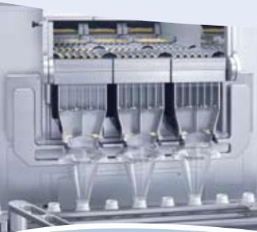
Mechanically controlled capping unit
