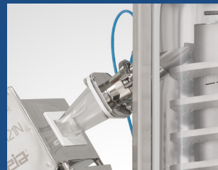
Dust-tight connection inclu- ding test tablet insert
