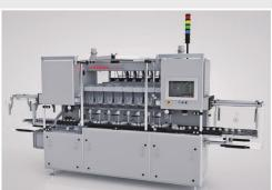
The CFI-622 counting and in-motion filling system comes in three different models for accommodating four, six eight CF-622 counting modules, depending on the required output.
