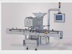
The CF-1220 is a 12-channel linear tablet and capsule counter with integrated bottle conveyor. The counter is specifically designed to be incorporated into complete packaging lines but is also very well suited as a stand-alone system.
