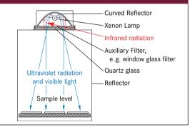
Spectrum: CIE 85/1989 SUNTEST with Daylight filter
